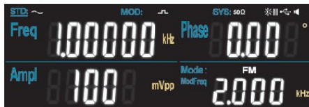
Picture 4-13 Set FM carrier waveform
